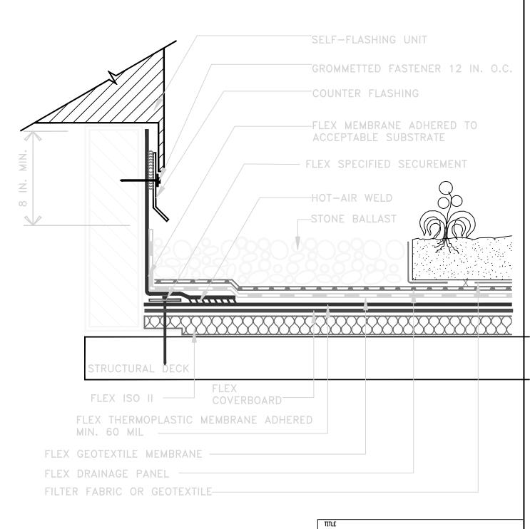
NOTE: MINIMUM 2 FEET OF BALLAST OF BETWEEN CURB AND GREEN ROOF
