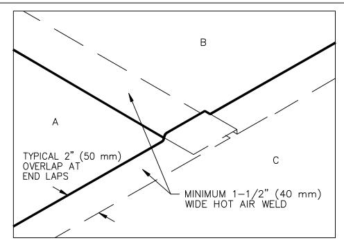
POSITION SHEETS AND HOT AIR WELD THE FLEX FIELD MEMBRANE A MINIMUM OF 1-1/2 (40 mm) INCHES.
