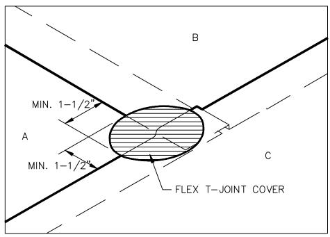
HOT AIR WELD A 4.5" DIAMETER FLEX T-JOINT COVER CENTERED OVER THE SPLICE INTERSECTION ("T-JOINT") AS SHOWN.
