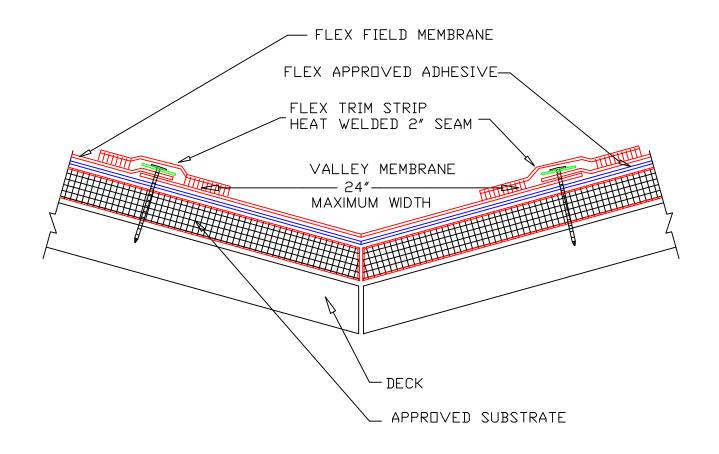
NDTE: FLEX TPD: FLEX TPD CUT EDGE SEALANT IS REQUIRED ON ALL NON FACTORY CUT EDGES OF FLEX TPD
